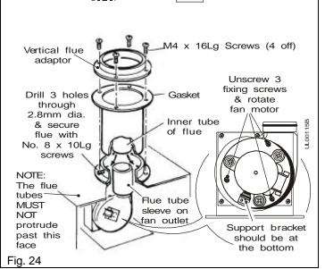
Retain the adaptor for connection of the flue system to the boiler.
